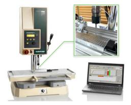
Test condition Testing bar : A7075 Tapping depth : 12 mm Hole diameter : 3.3 mm
